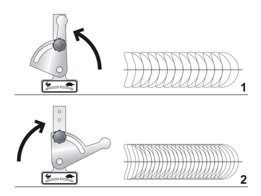
To either increase or decrease the rewinding speed intervene on the cam gearbox. To perform this stop the sprinkling system by stopping the water feed; then remove the actuating lever (*fig. D, pos. 2*) and screw, by means of a setscrew wrench (*fig. O, pos. 27*), the screw (*fig. O, pos. 28*) located on the cylinder with bearings.
