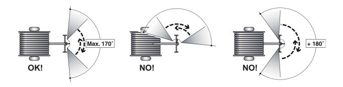
N) Lift the rings (1) by selecting the wished circle sector and tighten the screw (2).
