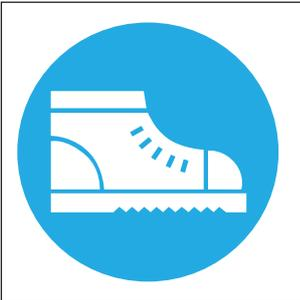
Wear safety shoes (with steel reinforced toe-cap).
